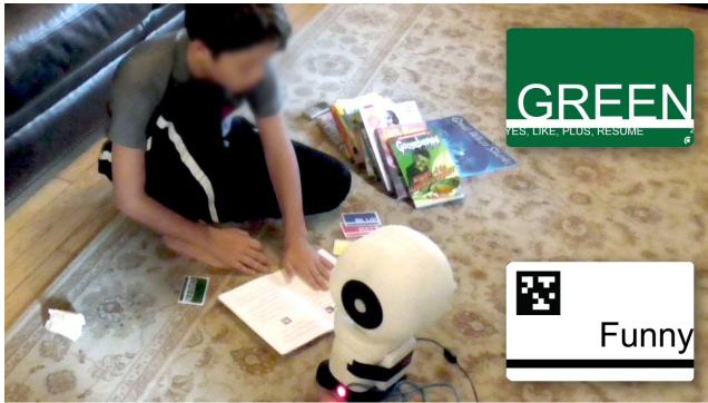
Figure 3. Image of a child working with Minnie during the introductory process. The child is holding a topic interest card and has placed the “Talking with Minnie” book on the floor in front of Minnie. The books available for the child to read appear on the right of the image. An example of a green RFID card (top) and a topic interest card with an April tag (bottom) are superimposed on the right of the figure.
