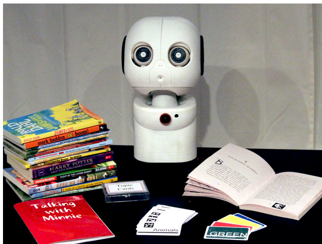
Figure 2. Image of the learning companion robot, Minnie, used in the study as well as the introductory "Talking with Minnie" book, RFID topic and interaction cards, and books augmented with AR tags. The robot's camera is the red circle on the upper torso. The RFID reader is below the camera and indicated by a red light when the robot is on.
